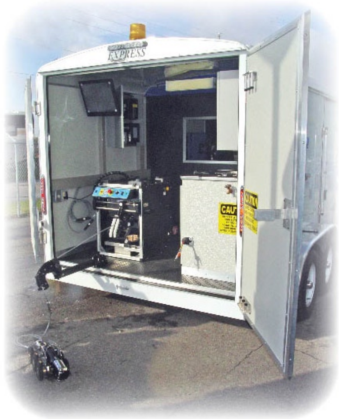
K2 Portable Inspection System - Trailer-mounted
