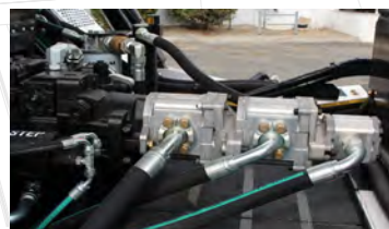
BELOW Elevator Type: optional 11 Flight squeegee with replaceable corded rubber tips; Continuous molded rubber belts combined with optional triple pump option (below) makes Global M4 CNG the ideal choice for sweeping heavy debris such as road millings, up to 3-tons per-minute. Standard leaf gate system assists in picking up large debris, bottles, large branches and leaves.
