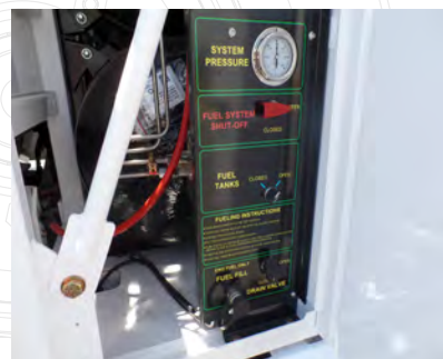
ABOVE Optional Reserve Tank Allows the operator to change the fuel source from the main tanks to the reserve tank through a keyed electrical switch.
