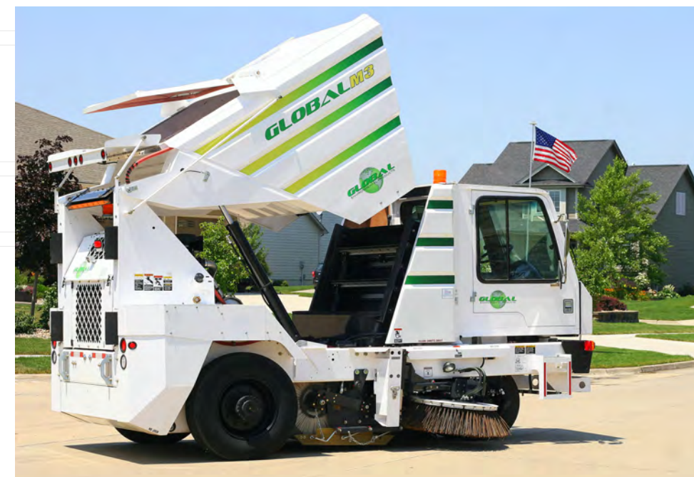
ABOVE The Global M3 is designed to make routine maintenance easy, so your sweeper spends more time on the street and less time in the garage. Two swing-out center body panels provide unrestricted access for elevator adjustment, maintenance and daily cleaning.
