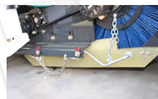
ABOVE Polyurethane Dirt Shoes will never damage while sweeping and last well above 1000 hours
