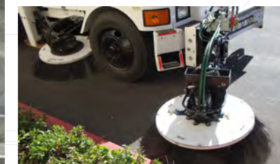
ABOVE Optional Front Articulating brush allows for extra reach to shoulders and center islands. Via In-cab joystic, the articulating front brush can be positioned on left or right side allowing for sweeping on right or left without changing seating positions.
