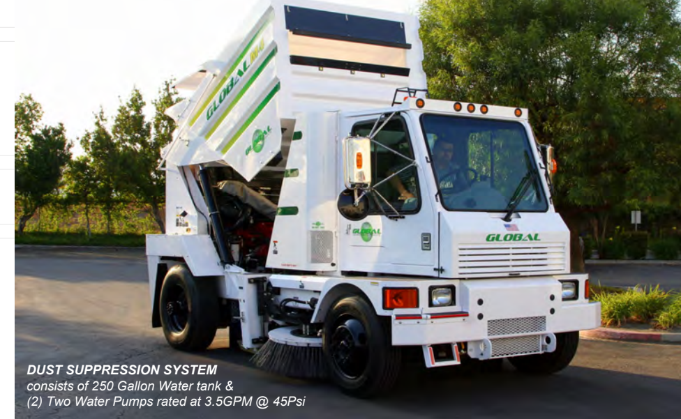
ABOVE The Global M4 is designed to make routine maintenance easy, so your sweeper spends more time on the street and less time in the garage. Two swing-out center body panels provide unrestricted access to elevator adjustment, maintenance and daily cleaning.
