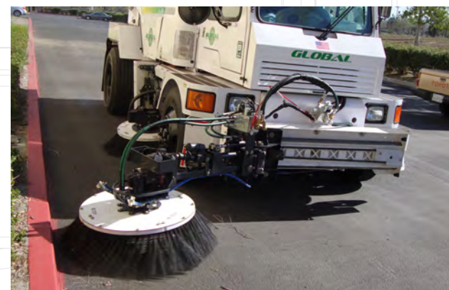
LEFT The Global M4 offers the best maneuverability in its class with its tight turning radius that allows the operator to maneuver easily in cul-de-sacs and close quarters.
