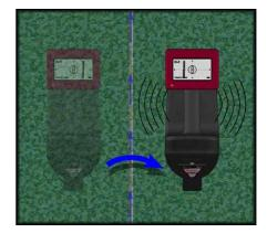
(d) Continue to walk away from the hook-up point, keeping the "line" on the screen under the center crosshair. If you wish, you may "wag" the pointer head side-to-side; this will cause the crossover alert to sound off as you walk along the line, and helps you to trace without watching the screen.
