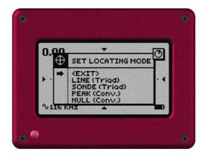
specific model type of the receiver ("SC", "UL", etc.). The various locating modes are listed and described here for reference.
