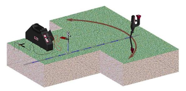
circle around the hook-up point. When the pointer head crosses over the line, the receiver will make a distinct alert sound (crossover sound). This, with graphic feedback on the LCD display,
