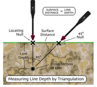
angle, move the pointer toward and away from the pipe, and narrow in on the precise null location. Mark this spot.
