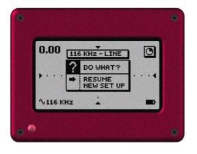
At the top of the screen you will see a memory strip indicating the most recent device set up (i.e., that was used on the previous locating job). At this time, you may either continue to locate with the stored settings (RESUME), or opt for new settings (NEW SET UP). Notice that a small timer icon appears in the upper right corner of the screen. When this graphic "times-out", any active menu will be removed from the screen, and the receiver will return to its original operating settings.
