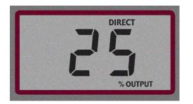
Select button to advance to it. Then use the Up or Down button to select a higher or lower output level. The available output levels are: 10%, 25%, 50%, and 100%. To the left is a typical screen one would see while adjusting the output level. Using the PULSE button
