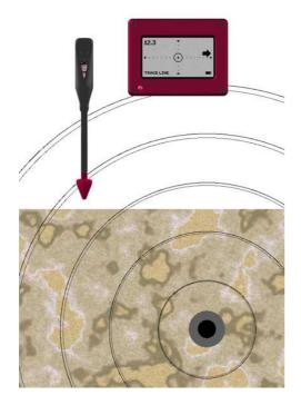
current-carrying line itself. The receiver determines the location of the actual line based on measurements made by the detection antennas.
