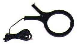
Advantages: no electrical contact point needed; very effective at energizing the target line only, even in congested areas. Disadvantages: part of line must be mechanically exposed enough to get clamp around it; limited target line diameter (up to about 5.5" OD).
