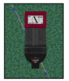
(c) When reporting the depth, the receiver requires a few moments to arrive at its most accurate result. Hold the receiver steady over the underground line until the depth report has stabilized.
