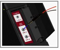
(c) Connect the black lead to a metallic stake that has been securely plunged into the ground. The amount of current generated on the target line depends largely on the nature of this ground connection. For longer traces, place the ground stake as far away from the red clip as possible. If little signal is required for the tracing job, then the user can even leave the black lead unattached and laying on the ground some distance from the red lead. This is referred to as an "off-ground" condition.
