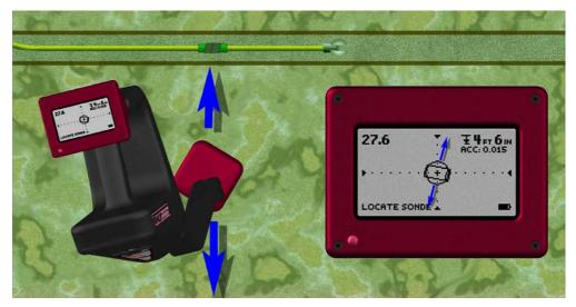
rectangle (or nearly so), the user should swing the pointer along the line that cuts through the middle of the icon. Move the pointer along this line, searching for the maximum ANR and/or the minimum depth report. When the receiver is so positioned, it will be pointing directly at the sonde.
