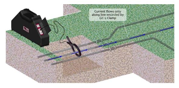
To use the GC-2 Clamp, simply plug it into one of the DIRECT output jacks (*SIGNAL[1]* or *SIGNAL[2]*), and encircle the target line with the clamp. Activate the 23X transmitter, and select the tracing frequency. It is recommended to use the clamp with RF frequencies only (33 KHz and higher). Only the line(s) enclosed inside the clamp will be energized.
