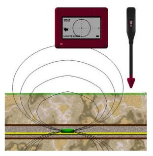
The Triad 2310 Receiver employs a unique technology to determine the location of the sonde. This technology allows the user to know immediately the location, depth, and orientation of the sonde. The technology is unlike traditional "peak and null" methods for sonde locating in that it does not rely on the use of a directional antenna to find tell-tale points around the sonde. Therefore, the technique is not limited by unusual or unanticipated orientations of the sonde.
