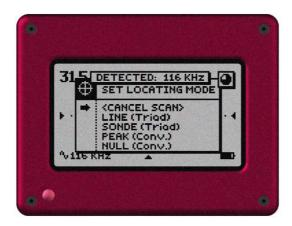
Having detected a signal from an active transmitter, the receiver will automatically present the "SET LOCATING MODE" menu. To continue, follow the instructions for setting the locating mode given on the following page of this manual. If you are unable to SCAN successfully, please refer to Appendix C, "Troubleshooting", for more help.
