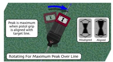
(d) Having thus aligned the receiver, mark the spot on the ground directly below the pointer antenna. Now move forward and/or backward from that spot to locate peaks at other spots over the line. As you traced the peaks, you will be tracing the course of the line.
