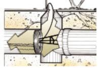
not to be used in restraining pipe plugs. These eyelets, rings and metal eyes are designed only for lifting and lowering of the plug.
