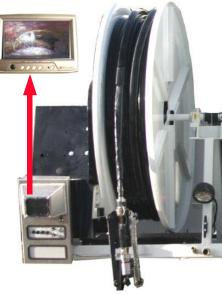
Patented Telescoping/ Rotating Dual Hose Reel is stored in the heated rear compartment and hydraulically extends out of the compartment using the new Ultra-Glide system for increased durability. The hose reel is also capable of 180 degree rotation. The Series II 800-HPRTV is now available with an optional hydraulically powered rotating hose reel.
