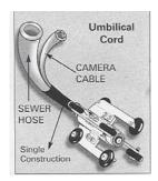
Umbilical Cord<sup>\*</sup> is a single unit construction of 5/8" sewer hose and multi-conductor camera cable wrapped in a protective, repairable molded casing. The 500' Umbilical Cord allows for easy jet tv operation working just like a sewer cleaning nozzle.
