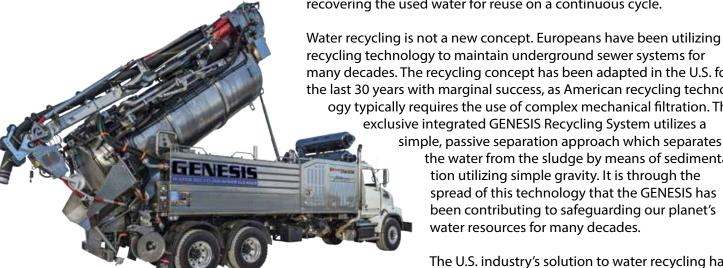
recycling technology to maintain underground sewer systems for many decades. The recycling concept has been adapted in the U.S. for the last 30 years with marginal success, as American recycling technology typically requires the use of complex mechanical filtration. The exclusive integrated GENESIS Recycling System utilizes a
